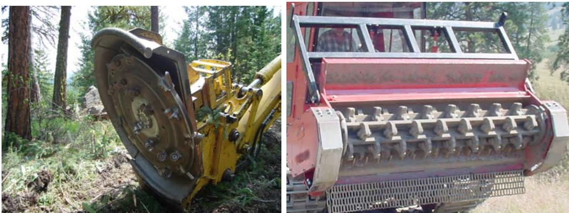
**Figure 2.** Examples of mastication heads. Vertical shaft (left photo) and horizontal shaft (right photo).
