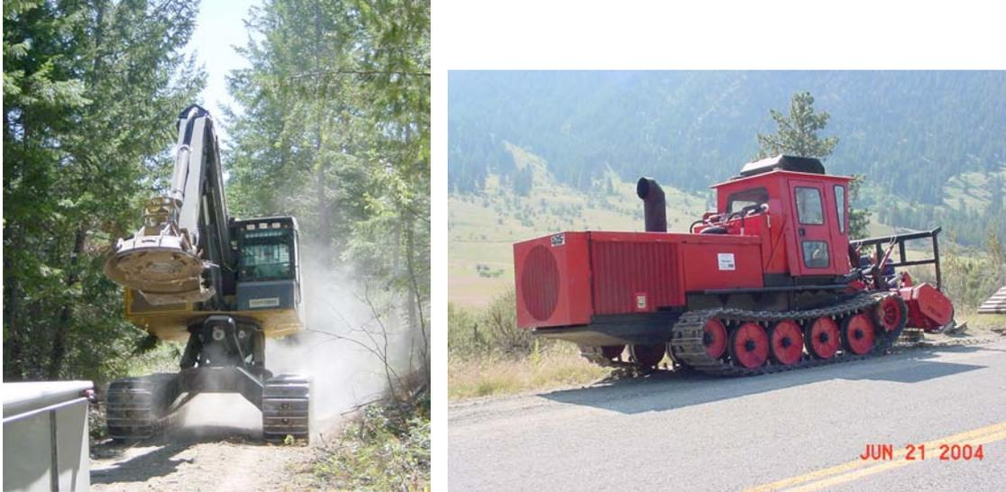
**Figure 3.** Examples of types of equipment commonly used for vertical shaft heads. Vertical shaft head mounted on self-leveling excavator (left photo) and rotary head fixed on tracked vehicle (right photo).
