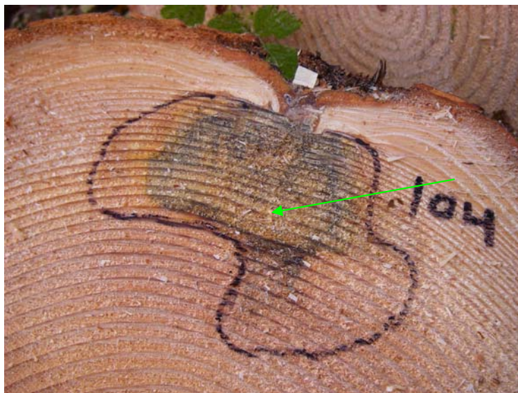
Figure 4. Purplish staining and softening of wood fibre (at green arrow) caused by P. pini inoculation.
