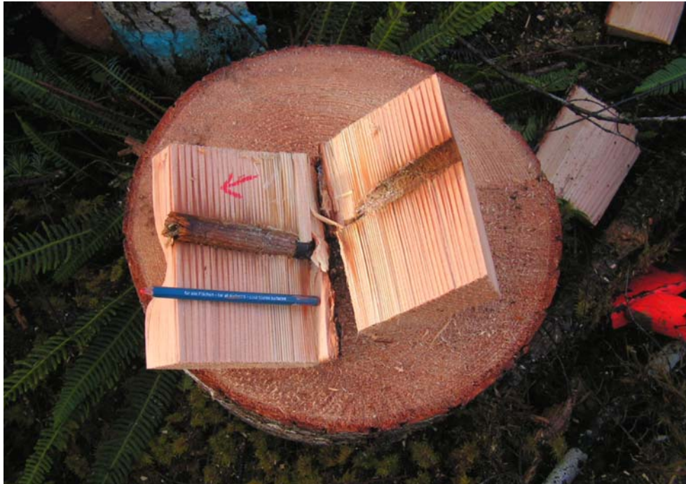
Figure 6. Tree destructively sampled in 2004 (one year post-treatment) showing early signs of decay (reddish-brown staining) in the heartwood surrounding the 4” dowel inoculation court. Red arrow points to the area of staining.
