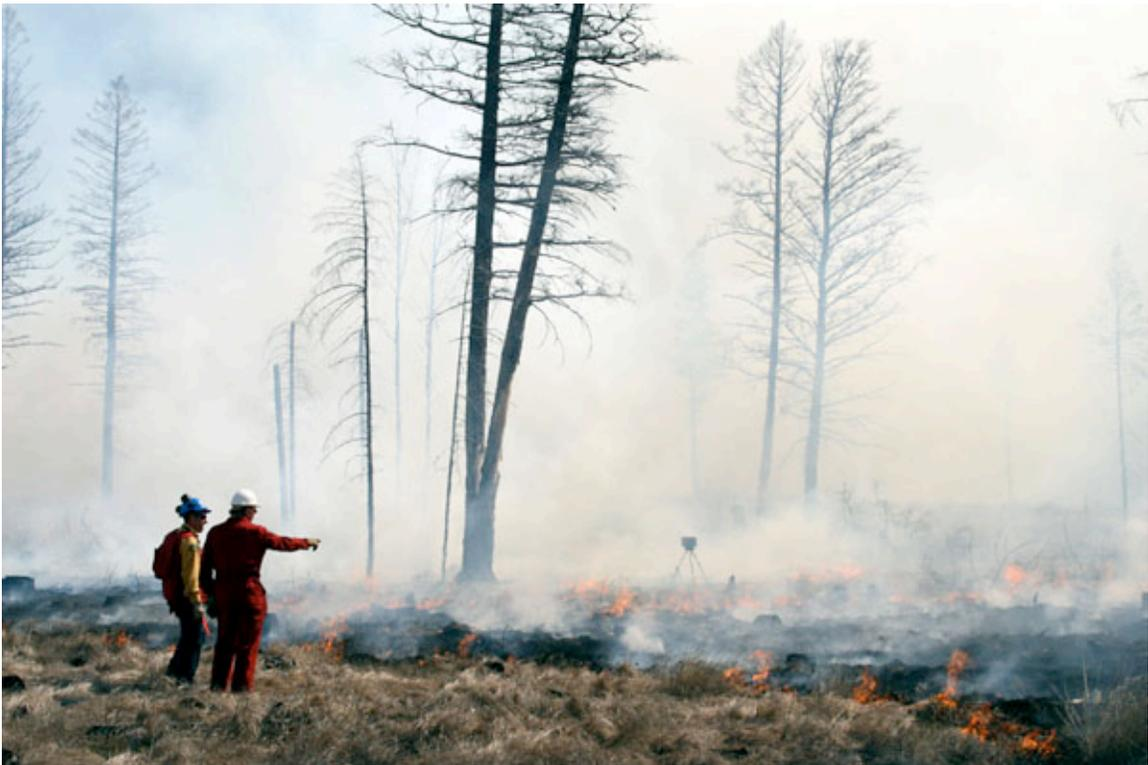
At centre is one of six video cameras mounted on tripods to record fire behaviour during the Redstreak Meadow prescribed burn.
